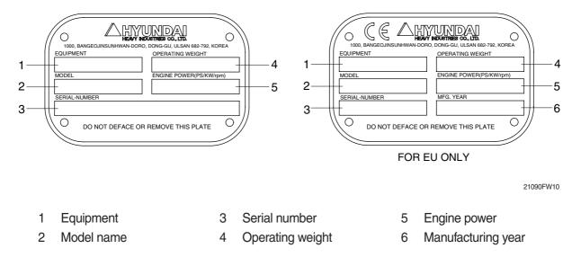
\* The machine serial number assigned to this particular machine and should be used when requesting information or ordering service parts for this machine from your authorized HYUNDAI dealer. The machine serial number is also stamped on the frame.
